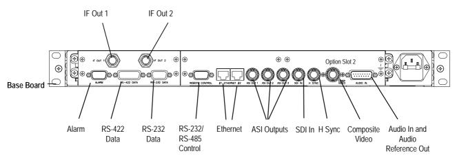
Figure 1.11: E5715 (1U) Rear Panel Component Parts and Connectors
